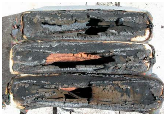
Figure 5. Fire-Blocking Layer; Horizontal Cushions
