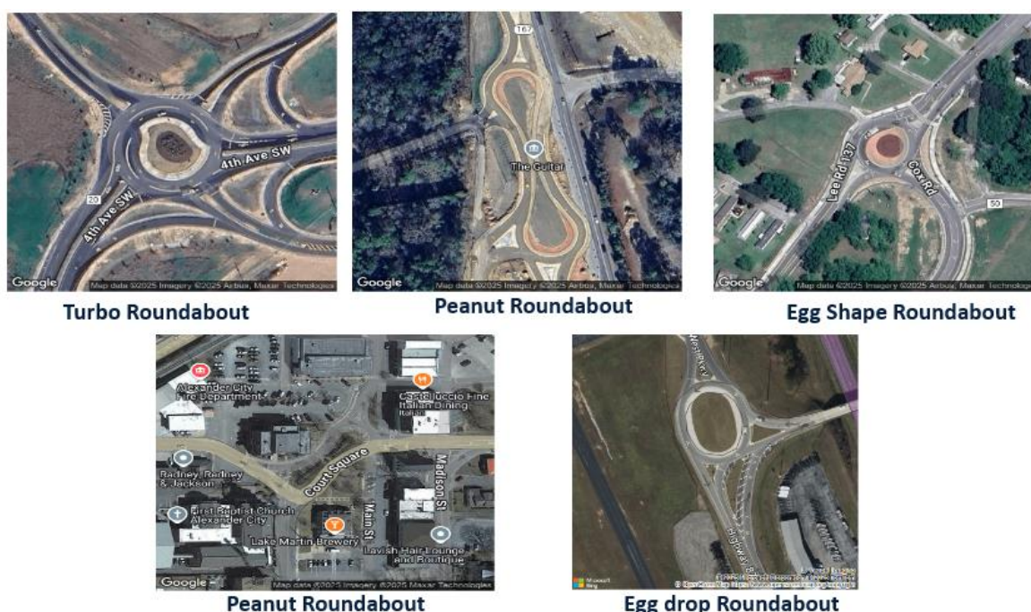
Figure 3-2 Non-Circular Roundabout Layout
