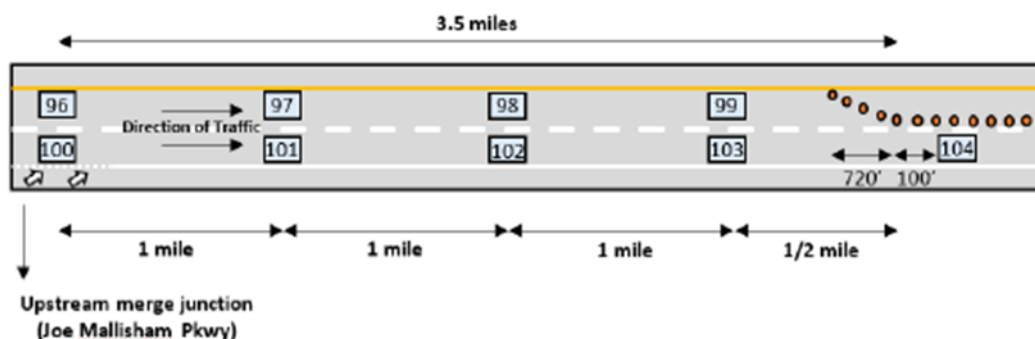
Figure 3-8 Traffic Sensor Deployment Scheme
