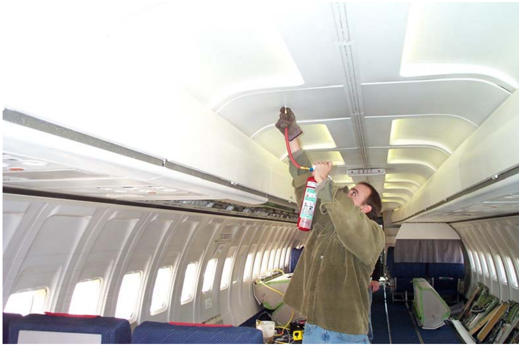
Figure 21. Halon 1211 Discharged Through Ceiling-Mounted Port
