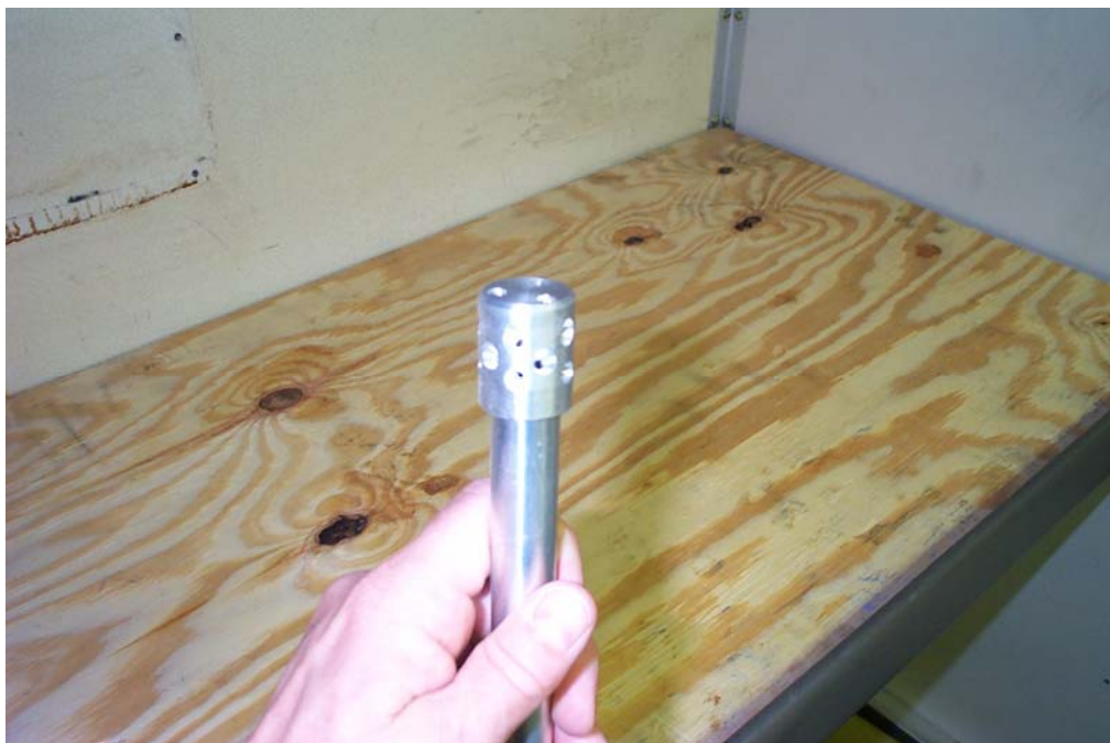
Figure 8. Ceiling-Mounted Port Prototype Discharge Head
