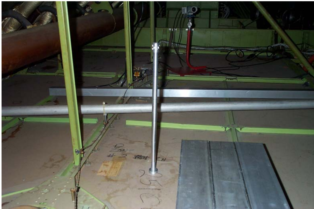
Figure 7. Ceiling-Mounted Port Extension Tube Mounted in Cabin Ceiling
