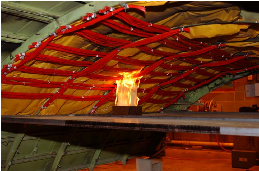
Figure 1. Wiring Test in a Simulated Cabin Overhead Area
