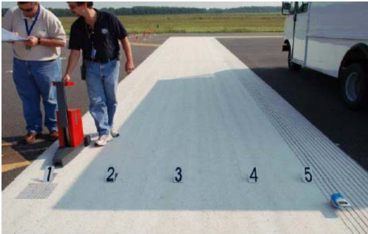
Figure 6. Airport Safety Technology R&D Sub-Team Members Taking Retro-Reflectivity Readings
