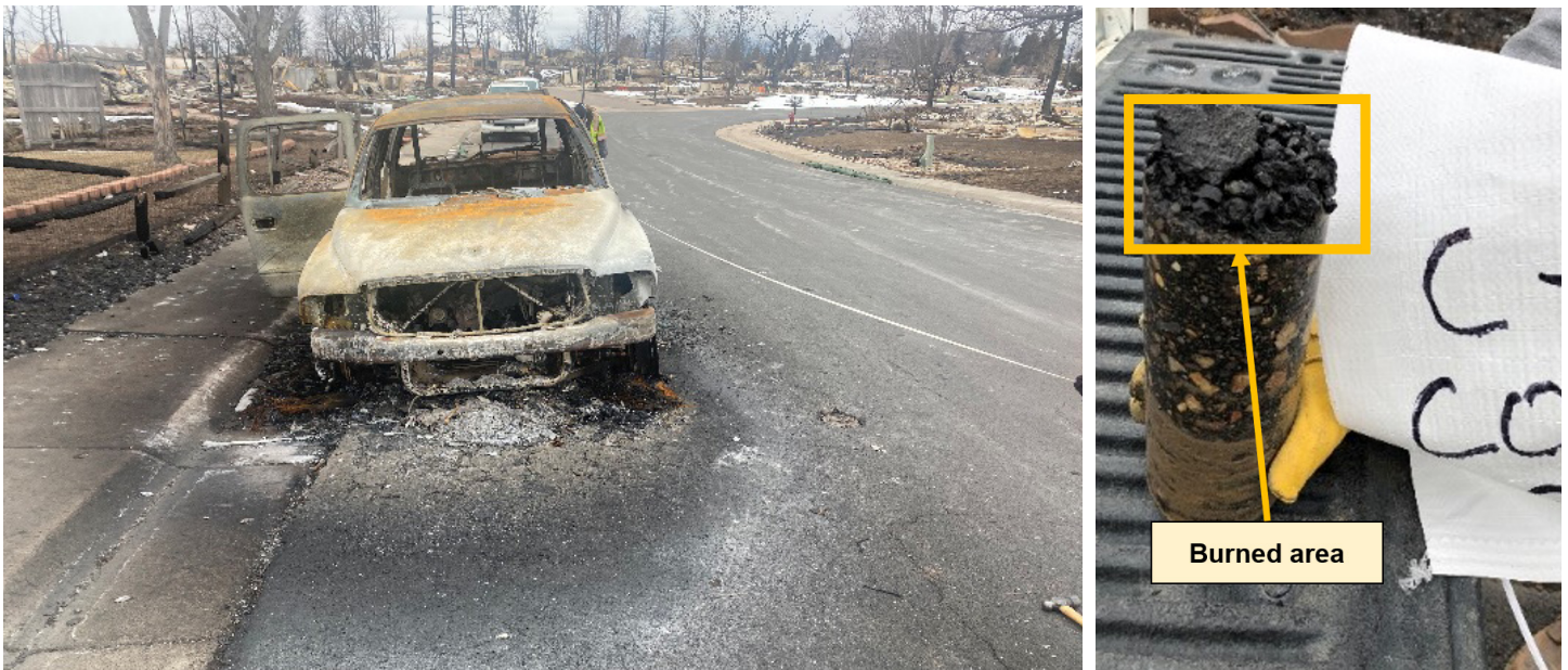
A. Burned pavement from car.
