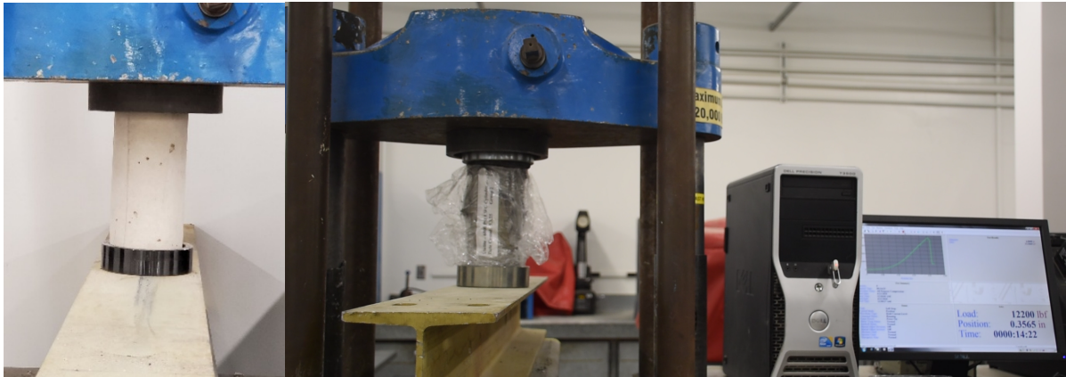
Figure 22. Compressive Strength Sample (Left) and Testing (Right)
