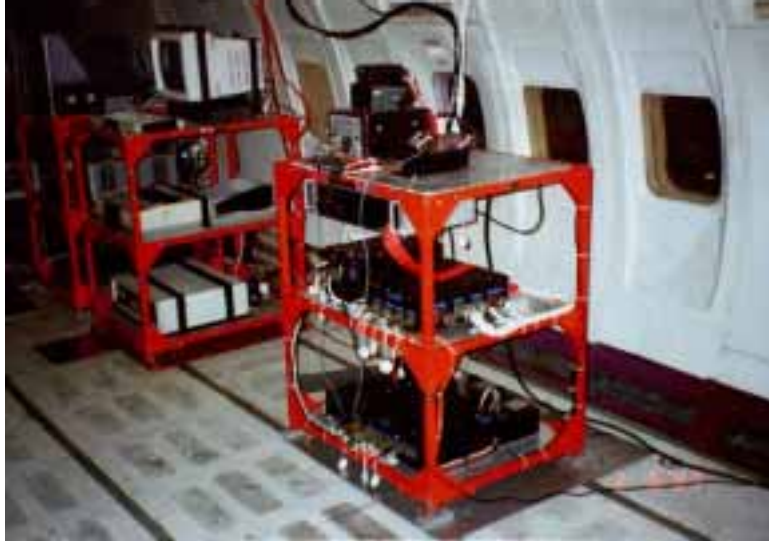
FIGURE 3. B-727 ONBOARD DATA ACQUISITION SYSTEM
