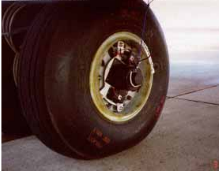
FIGURE 1. WHEEL WITH INSTRUMENTATION AND TIRE MOUNTED
