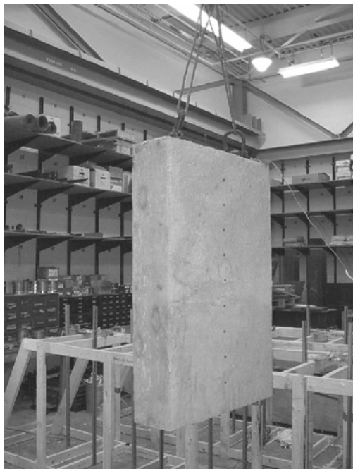
Figure 5.30: Transferring Deck Models to the Testing Frame
