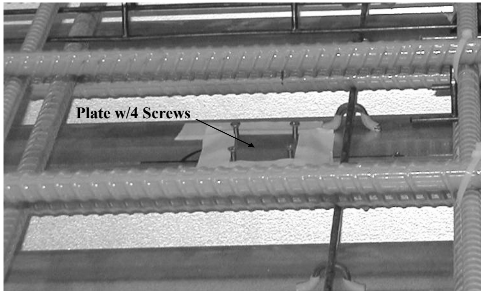
Figure 4.40: Steel Bonding Plate in As-Built Model
