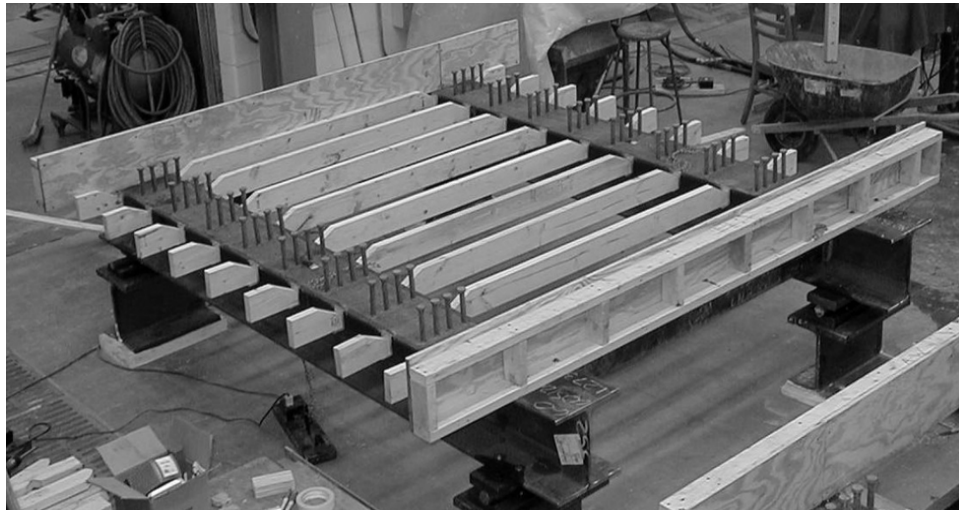
Figure 4.11: Joists Attached to Clips in Free-Shrinkage Model
