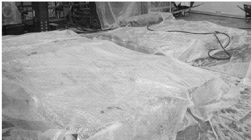
Figure 5.28: Deck Models Covered with Burlap and Plastic
