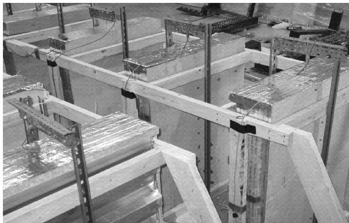
Figure 5.18: Testing Frame After Placement of Specimens and Instrumentation
