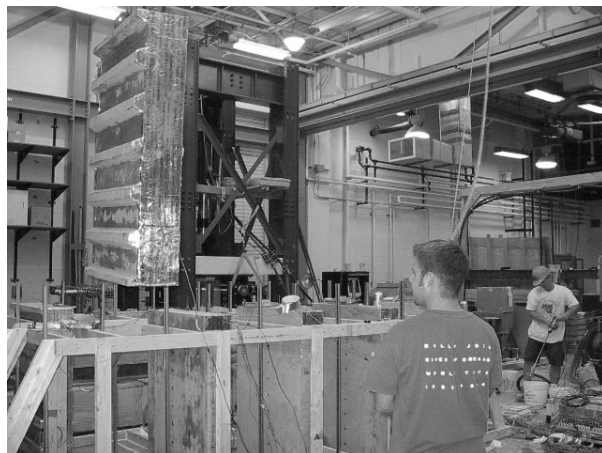
Figure 5.32: Installing Deck Models Into Test Frame
