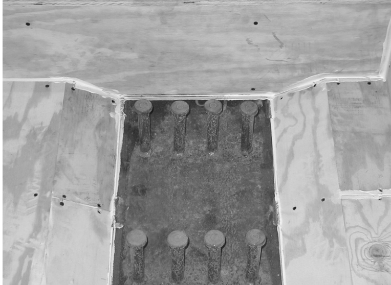
Figure 4.15: Fabricated Profile for Free-Shrinkage Model
