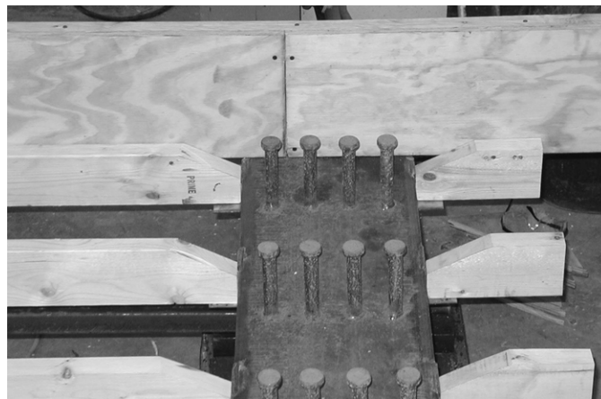
Figure 4.12: Angle on Ends of Joists in Free-Shrinkage Model
