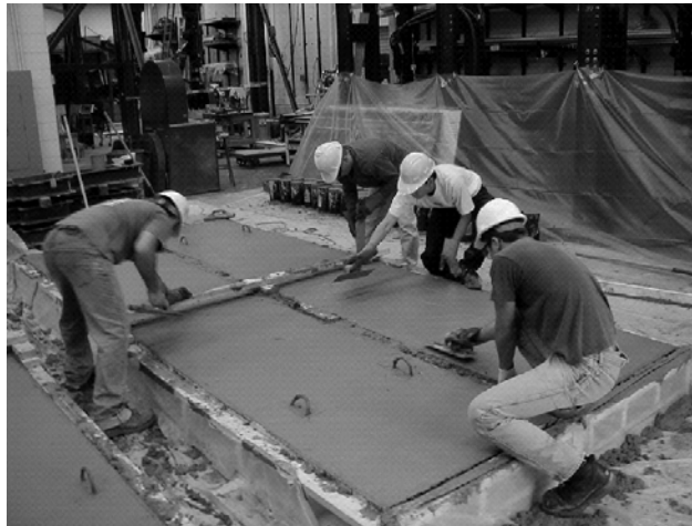
Figure 6.10: Finishing the Slab Specimens
