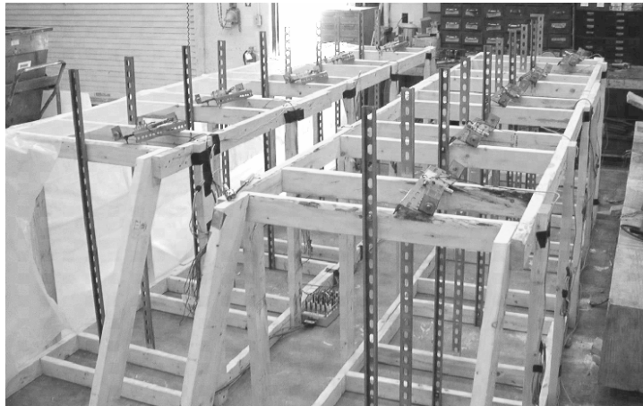
Figure 5.17: Testing Frame Before Placement of Specimens and Instrumentation
