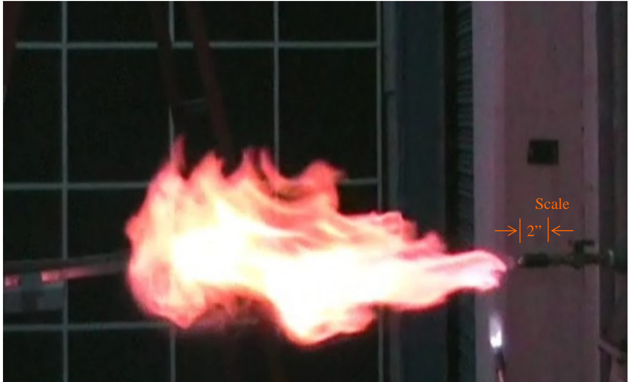
Figure 3. Observed Fire Plume From the Misting of TKS Anti-Icing Fluid in the Presence of an Ignition Source
