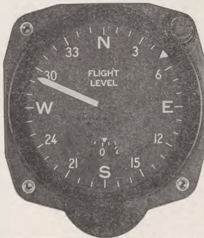
FIGURE 1.—The experimental flight level indicator developed by the Civil Aeronautics Authority.
