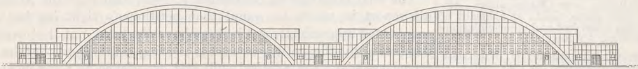
HANGARS ELEVATION FROM FIELD SIDE
