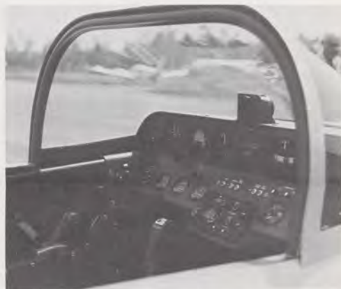
Pieper's grouping of his engine and propeller controls in one quadrant on the left side of the cockpit reflects his background as a military pilot. Instrumentation in his plane far exceeds basic FAA requirements.
