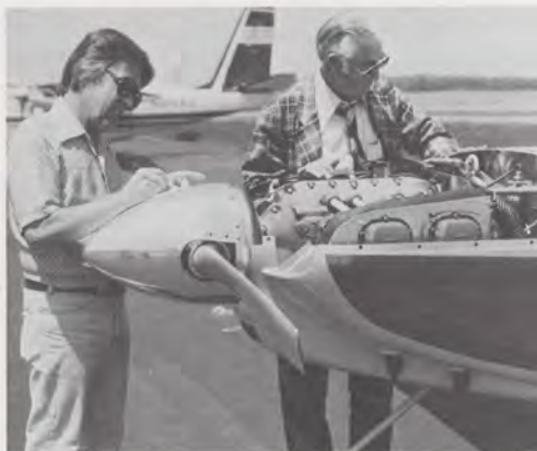
Will Pieper takes notes as inspector Ralph H. Moffitte from FAA's Harrisburg (Pa.) Engineering and Manufacturing District Office 44 probes the engine's oil and electrical systems and controls. No major deficiencies were uncovered. The craft easily won its Airworthiness Certificate.
