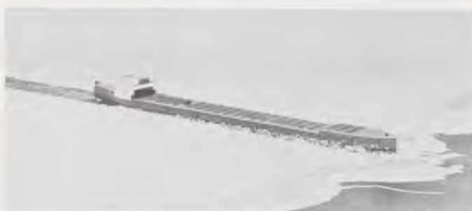
This scale model of a freighter is sailing through a make-believe sea covered with a wax-like chemical compound that simulates actual ice. The model is used by the St. Lawrence Seaway Corporation engineers studying the feasibility of keeping the seaway open 12 months of the year.
