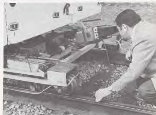
With the use of a portable ultrasonic testing unit, a technician at DOT's Transportation Systems Center (TSC) can readily detect the presence and character of a rail flaw, which is indicated and registered by a mobile inspection system. The demonstration took place at TSC's rail facility at Cambridge, Mass., and is part of the Federal Railroad Administration's continuing search for increased safety.
