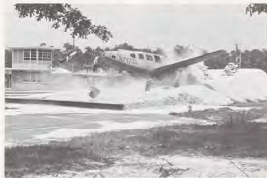
Fuel sprays from a ruptured conventional wing tank as a Piper Navajo simulates a crash landing in a test of fuel tanks at FAA's National Aviation Facilities Experimental Center, N.J. A two-ply rubber-coated fabric tank designed to FAA specifications in the left wing survived the impact. William Perrella is the project engineer, assisted by James Daily, Harry Hogg and Maurice Dungan. The plane was donated by Piper Aircraft Corp.
