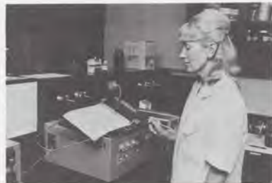
Mrs. Virginia Peterson interprets the infrared spectrum of an oil sample under analysis in the fingerprinting process.
