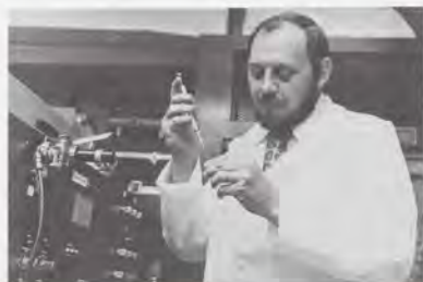
Harry Giles withdraws an oil sample for use in the gas chromatograph during one of the steps in determining an oil's fingerprint.
