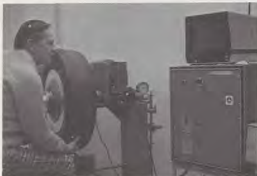
Henry Bessler, Transportation Systems Center, Cambridge, Mass., evaluating a tire casing using the ultrasonic inspection system developed by the Office of Vehicle Safety Research of NHTSA.
