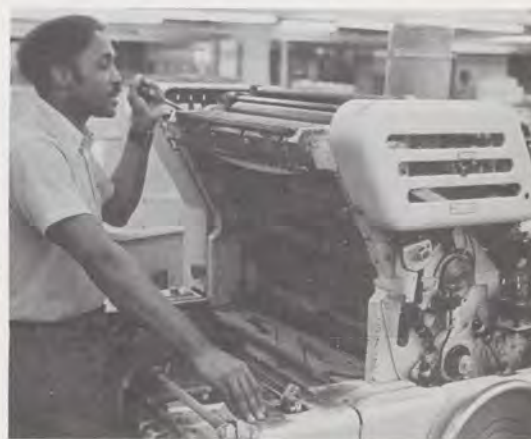
Neal Law keeps a vigilant eye on a big Harris 17x22 offset press. The P-2 plant has two of these presses which can handle jobs ranging from 8 inches by 10½ inches to 17 inches by 22 inches, producing up to four 8½ inch by 11 inch units with each pass through the press.
