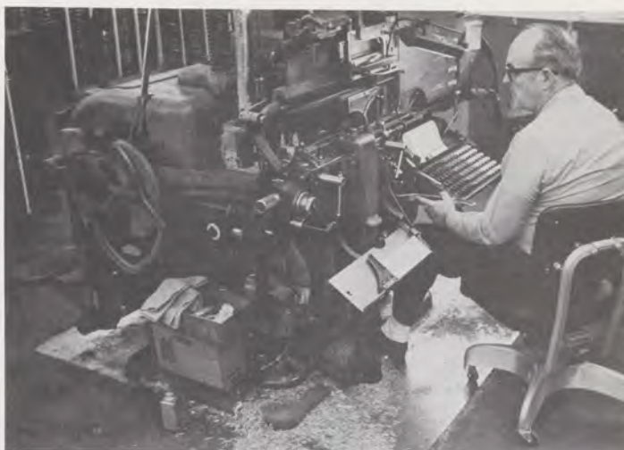
Don Lester at the keyboard of the Intertype slug casting machine. The machine converts molten lead into a wide variety of type faces and sizes. These words you are reading, for example, were cast on this machine.
