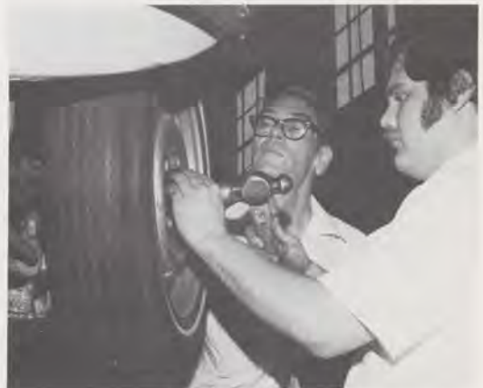
Close to the final station inspectors remove a wheel and bearing to determine its condition and to estimate the general status of the other wheel bearings. As a routine matter the wheel containing the speedometer linkage is pulled.
