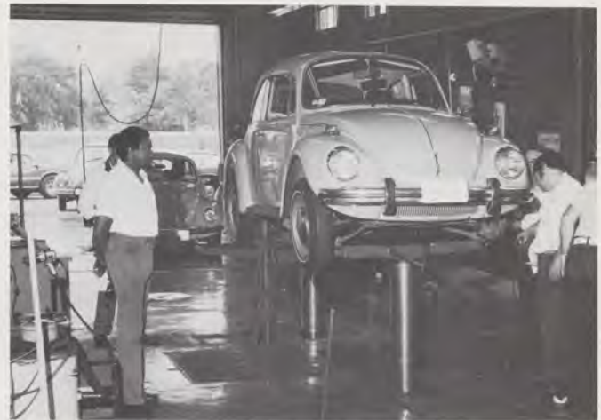
Following engine analysis the car is run on rollers at various "speeds" where brakes and general running characteristics are examined. The vehicle is then raised for an underside inspection.
