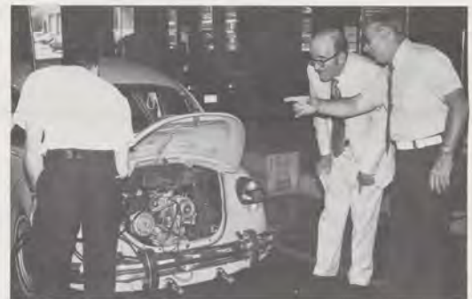
After passing the initial inspection station, where the car's oil and fluids for the battery, brakes, automatic transmission and windshield washer are checked, the car is connected with an electronic engine analyzer. Here the engine's electrical and fuel systems are checked, and samplings made of engine emissions. Dairi Bragg, program analyst for the Vehicle State Demonstration Program, explains the procedure to a visitor.
