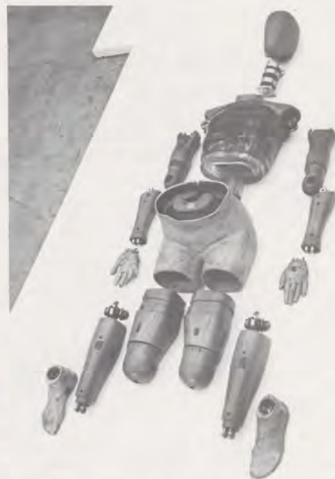
Oscar, the anthropomorphic dummy built to NHTSA specifications, plays a vital role in automotive crash research. Built-in electronic sensors and sending units can transmit precise data on every phase of a crash test. Oscar costs about $10,000.
