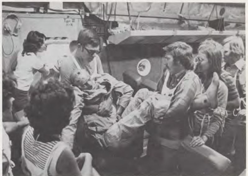
An "unconscious" dummy is carried toward the exit hatch during a drill in the evacuation simulator at the Federal Aviation Administration's Civil Aeromedical Institute (CAMI), Oklahoma City, Okla.
