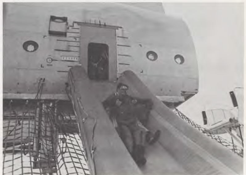
Researchers handle "handicapped" dummies being evacuated from a simulator as part of the test program. A wide variety of "disabilities" are studied so as to develop a broad range of experience.
