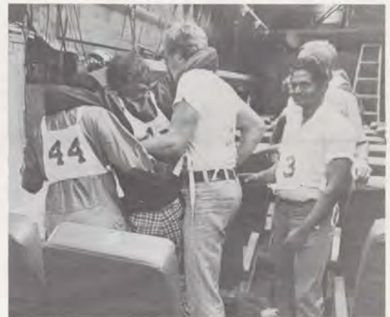
A researcher plays the role of a disabled passenger in a carefully set-up "crash" test. The simulator used in the project is a cast-off C-124 fuselage with an interior that can be modified to accommodate various air emergency scenarios. A discarded spiral staircase from a Boeing 747 is one of the test devices used.
