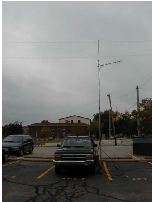
Figure D-4: Portable slave station with Yagi at two West Lafayette locations.
