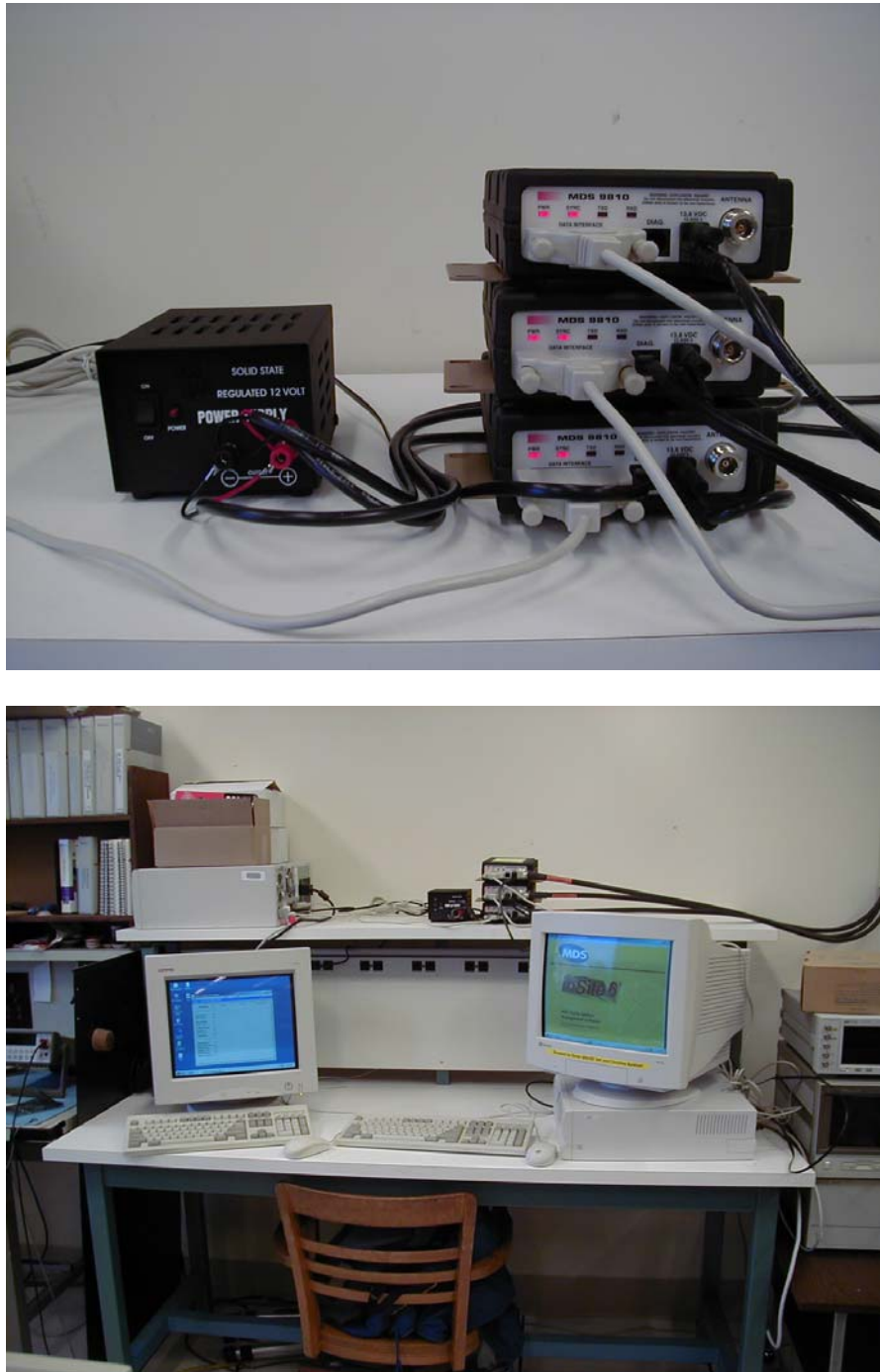
Figure D-1: (Top) View of three MDS 9810 spread spectrum radios in the WCRLab in the MSEE building. These radios are connected to three antennas mounted on masts on the roof of the building. (Bottom) View of computers used for radio control and RLTS software.
