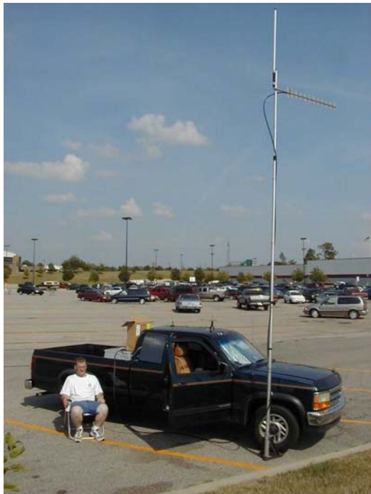
Figure D-4: Portable slave station with Yagi at two West Lafayette locations.
