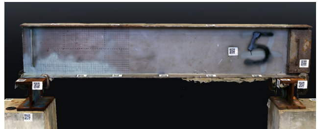
Figure 3.16 Horizontal Views of the Resulting 3D Models. Scanning Date: August 10, 2023, Refined Sparse Capture Strategy.
