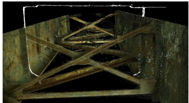
Figure 3.29 Compact Drone Scanning Result: 3D Reconstruction Result.
