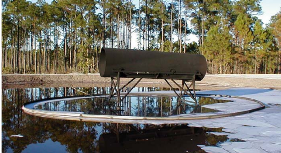
Figure 4. F-100 Engine Nacelle With 30-ft-Diameter Ring
