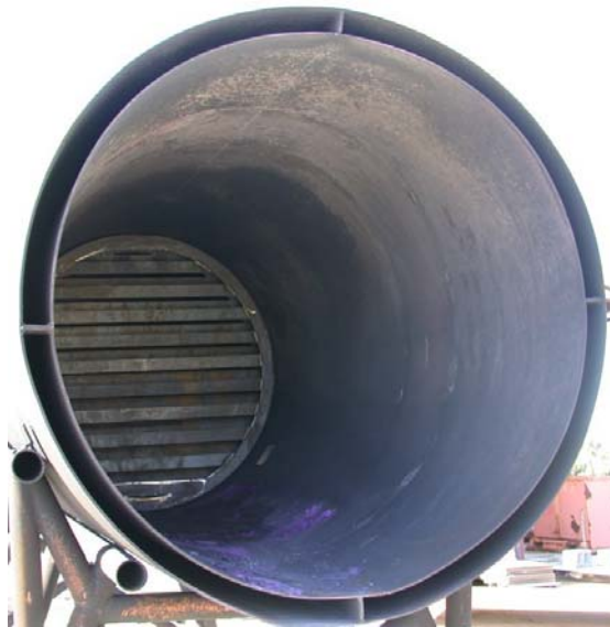
Figure 5. F-100 Engine Nacelle Metal Baffling Inside Nacelle
