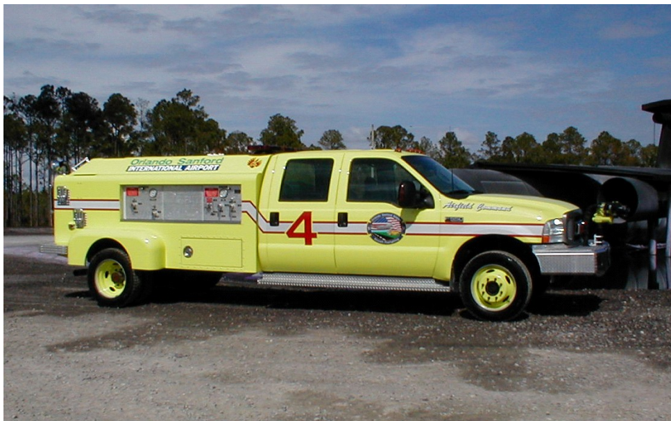
Figure 1. Quad-Agent Fire System
