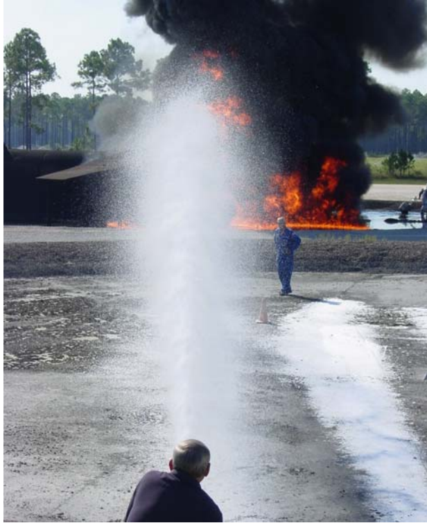
Figure 9. Discharge Distance AFFF Test
