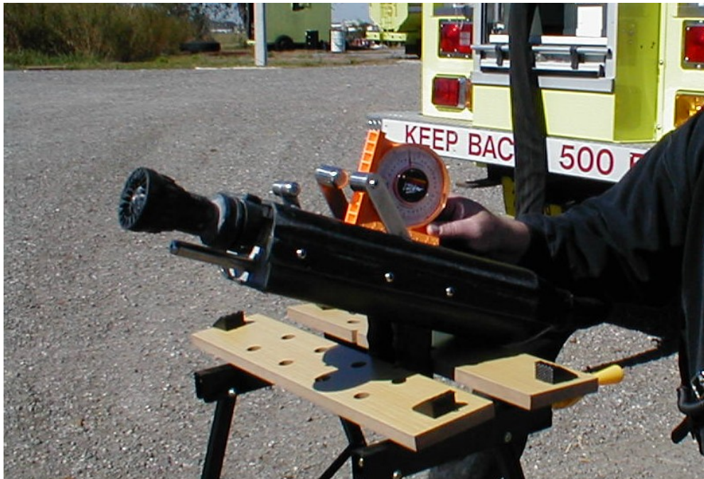
Figure 3. Hand Line Nozzle Mounted on Table for the Agent Discharge Distance Test
