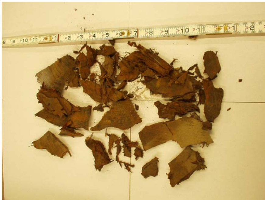
Figure 3.1 Tire Shreds Used for the Embankment
