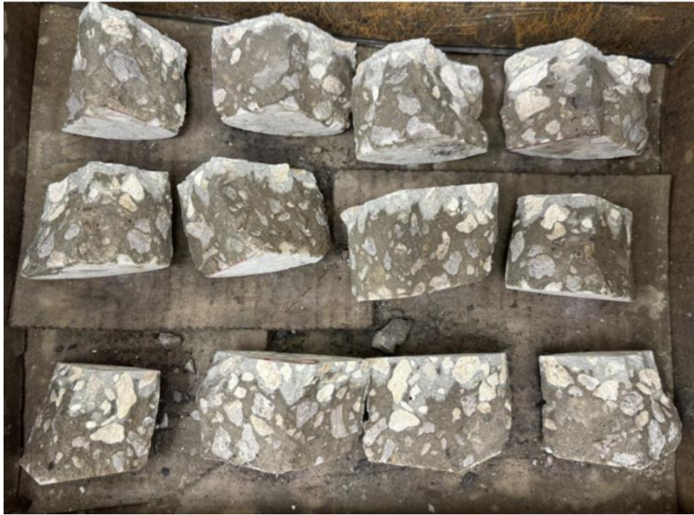
Figure 86. RMT samples after splitting
