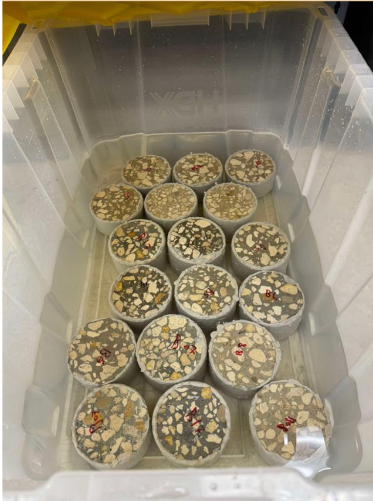
Figure 26. Samples inside the exposure tank
