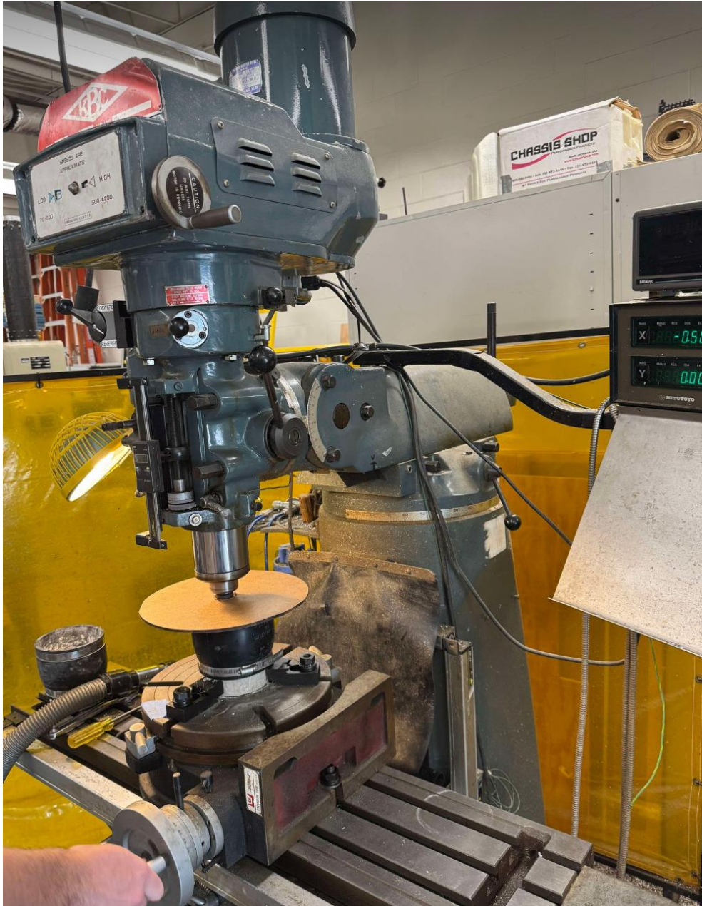
Figure 27. Grinding with concrete milling machine
