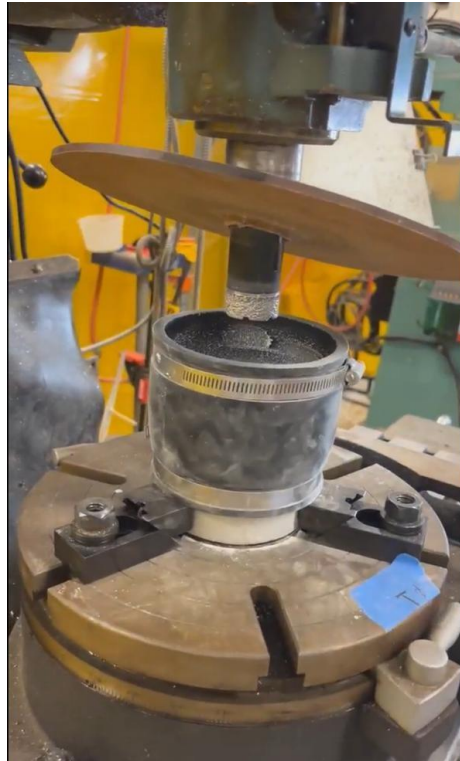
Figure 28. Concrete sample in position on milling machine stage
