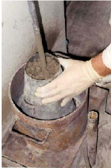
Fig. 7.3 Ve-Be cone top layer being filled
