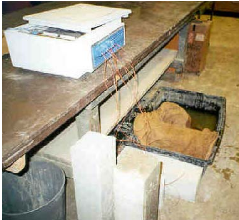
Fig. 8.1 Temperature in specimens being monitored by data-logger
