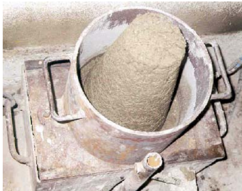
Fig. 7.4 Concrete specimen placed in the test mold on vibrating table right before starting the vibration
