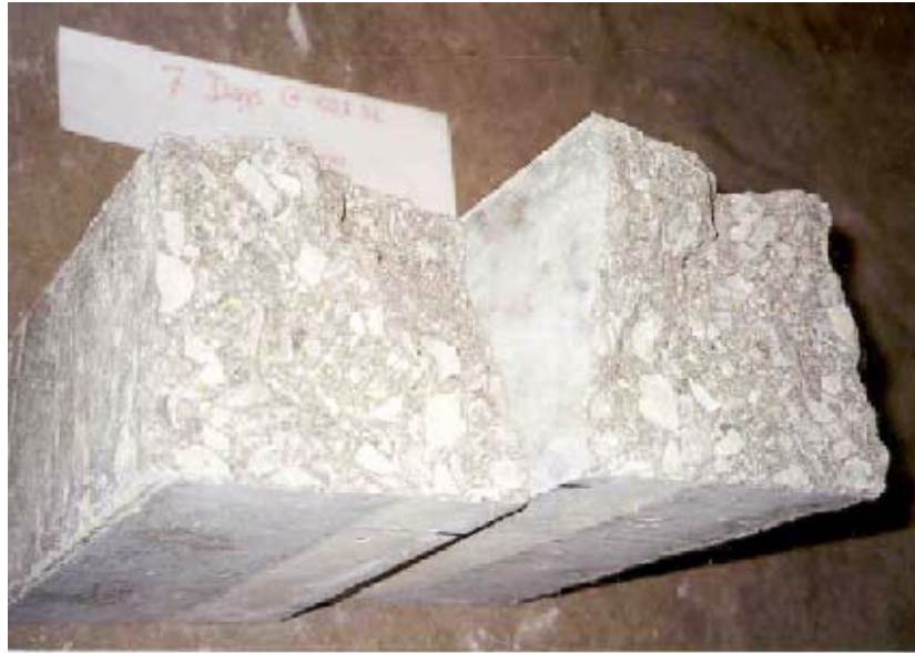
Fig. 8.14 Cross-section of a beam that failed at 3360 cycles at 90% stress level after 7 days of curing.
