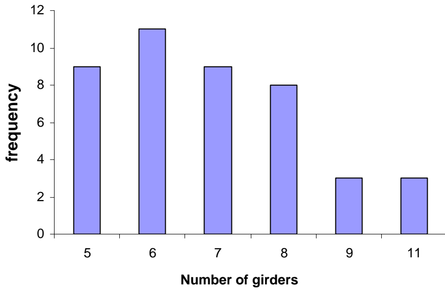
Figure 4.17 Representative Bridge Histogram (Number of Girders).
