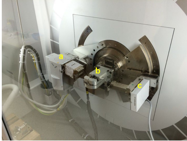
Figure 10. XRD System at UCF (a) X-Ray Tube; (b) Sample Holder; (c) Detector
