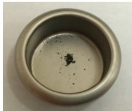
(b) Fragments of oxide layer
