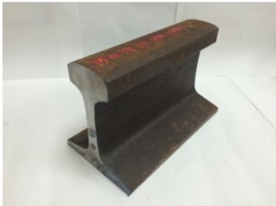
(e) 1948 rail (isometric view)
