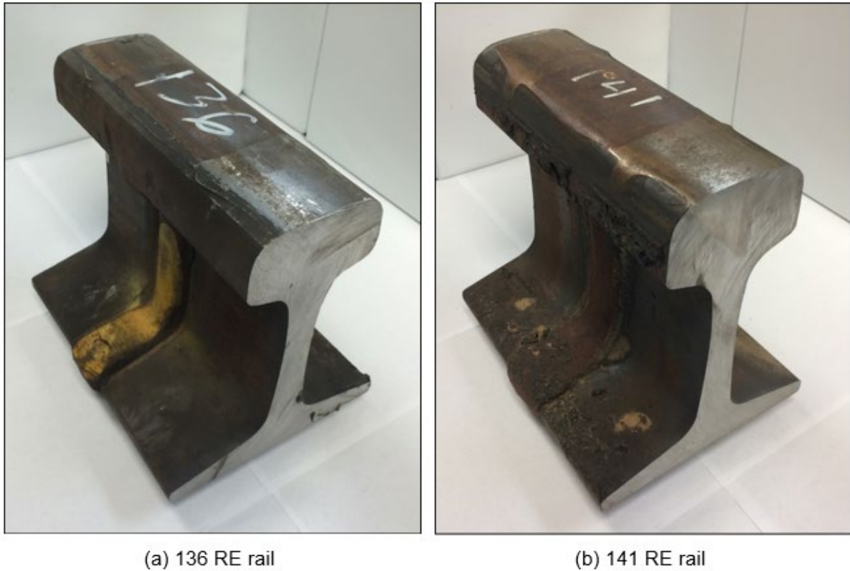
Figure 58. Photographs of thermite welded rails.
