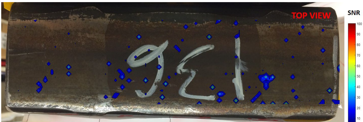
Figure 65. 2D intensity map of \alpha -Al 2 O 3 on the rail head (top view)
