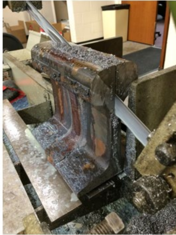
(b) Rail cutting
