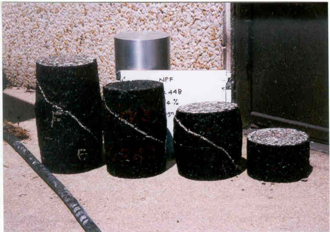
Figure 6.7 Observed Failure Planes for Different Height to Diameter Ratios.
