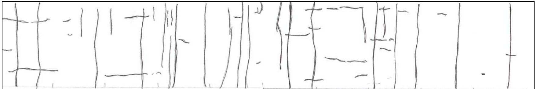
Figure 25b 1996 Cracking Pattern
