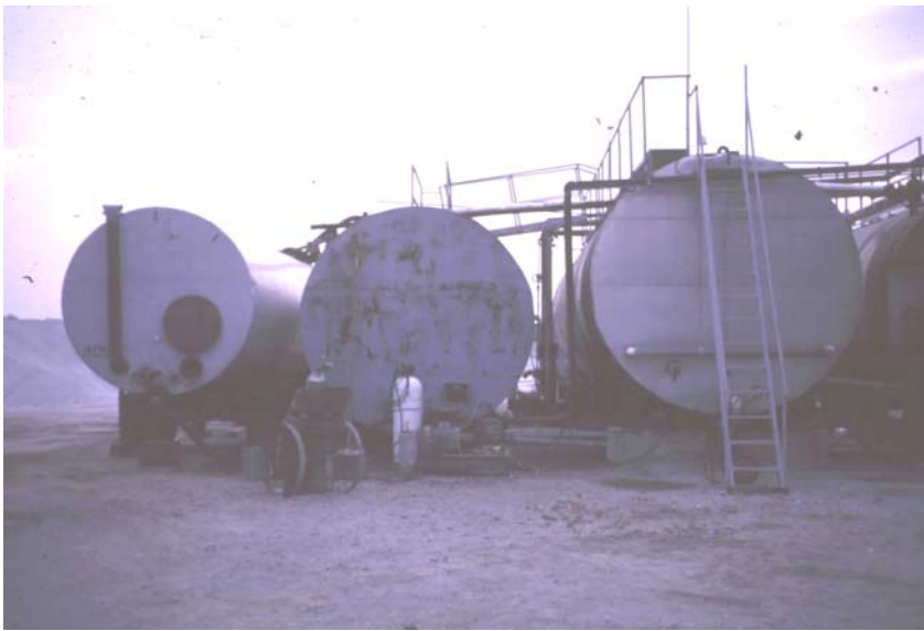
Figure 8 Neoprene, MGAC and PAC Were Metered into AC Line at Plant
