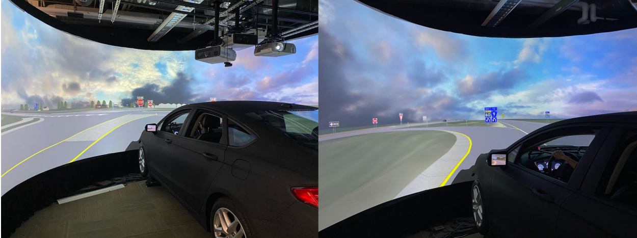
Figure 1. HFSL immersive driving simulator
