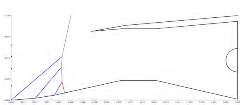
Figure 10. Example M=1.7 SST inlet experiencing external oblique-normal shock interactions (purple lines).
