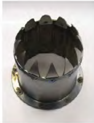
Figure 36. Chevron nozzle with removable chevrons from experimental study (Henderson & Bridges, 2010).
