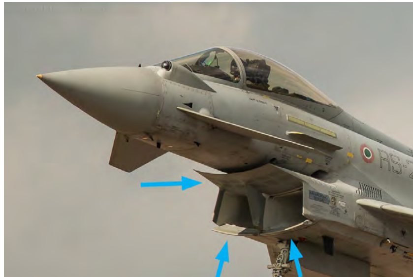
Figure 23. Eurofighter Typhoon VGCL inlet (Aircraft Recognition Guide, 2018).
