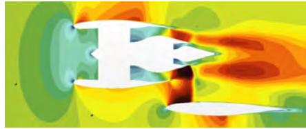
Figure 10. Mach contour plot shows influence of wing on exhaust streams of engine.
