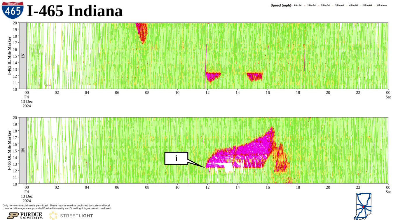
Figure 5.11 Traffic Speed Heatmap for Section of I-465 in Indiana from MM 10 to MM 20 on Friday, December 13, 2024.
