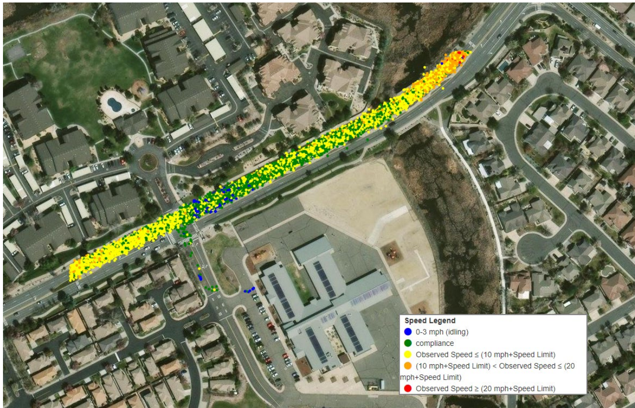
FIGURE 15: Speed Distribution across a School Zone extracted from Vehicle Telemetry Trajectory Data
