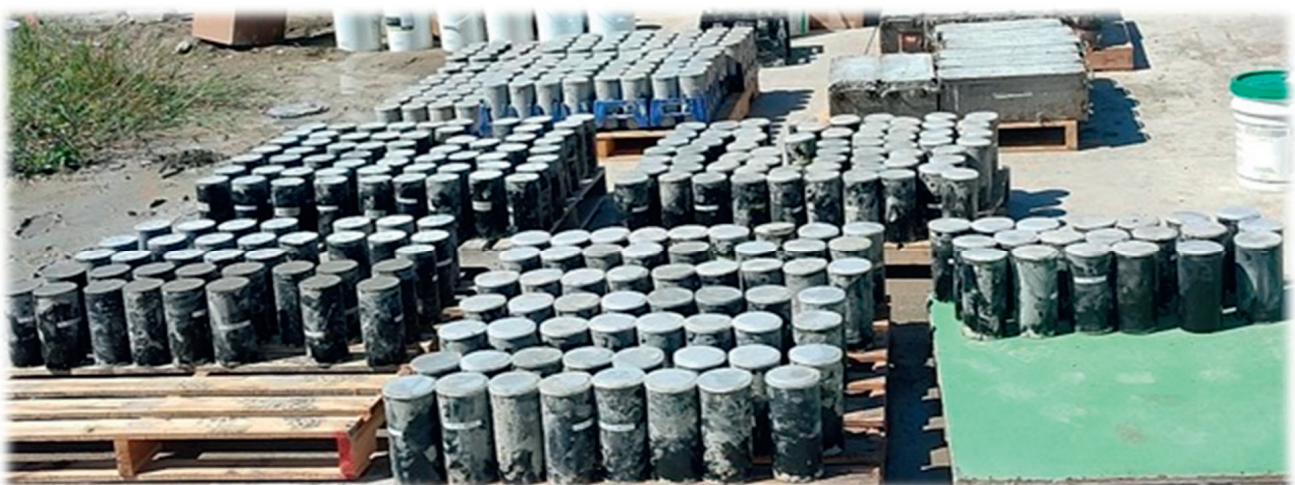
Figure 6.4 Field-Cast 4 × 8 in. Concrete Cylinders.
