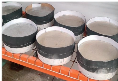
(d) Diked Specimen Ponded With Chloride Solution.
