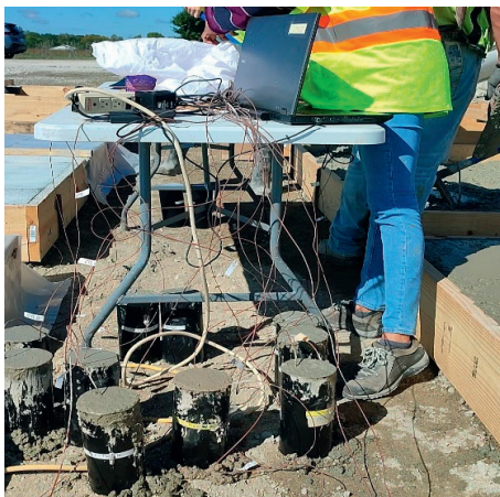
Figure 6.7 Thermocouples Embedded in Concrete Cylinders.
