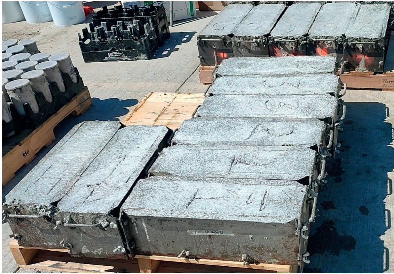
Figure 6.5 Field-Cast 6 × 6 × 18 in. Concrete Beams.
