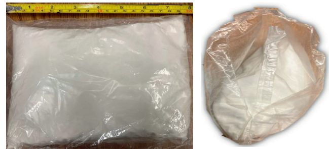
Figure 6.1 Dry SAP Particles in 8 × 6 in. Dissolvable Bags.
