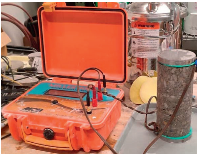
Figure 6.14 Test Setup for Concrete Resistance Measurements.
