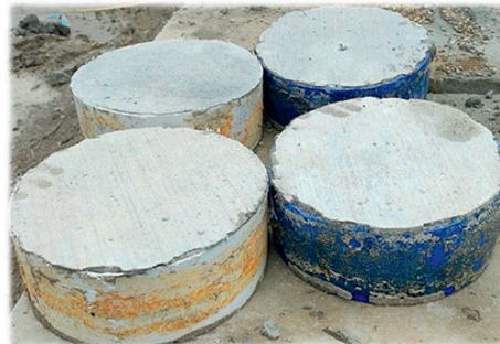
(b) Specimens for Scaling Resistance Test.
