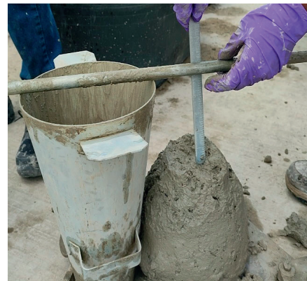
Figure 6.12 Evaluation of the Concrete Workability (Slump).
