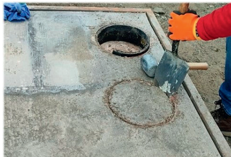
(a) Extraction of Test Specimen From the Field.
