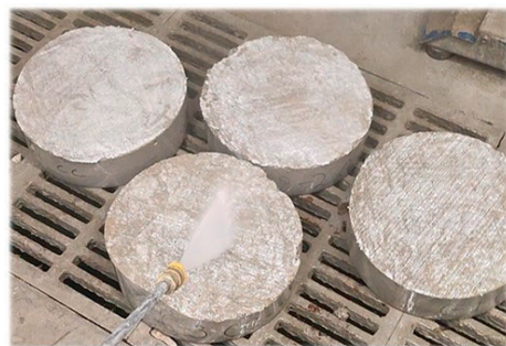
(c) Specimens for Scaling Resistance Test.
