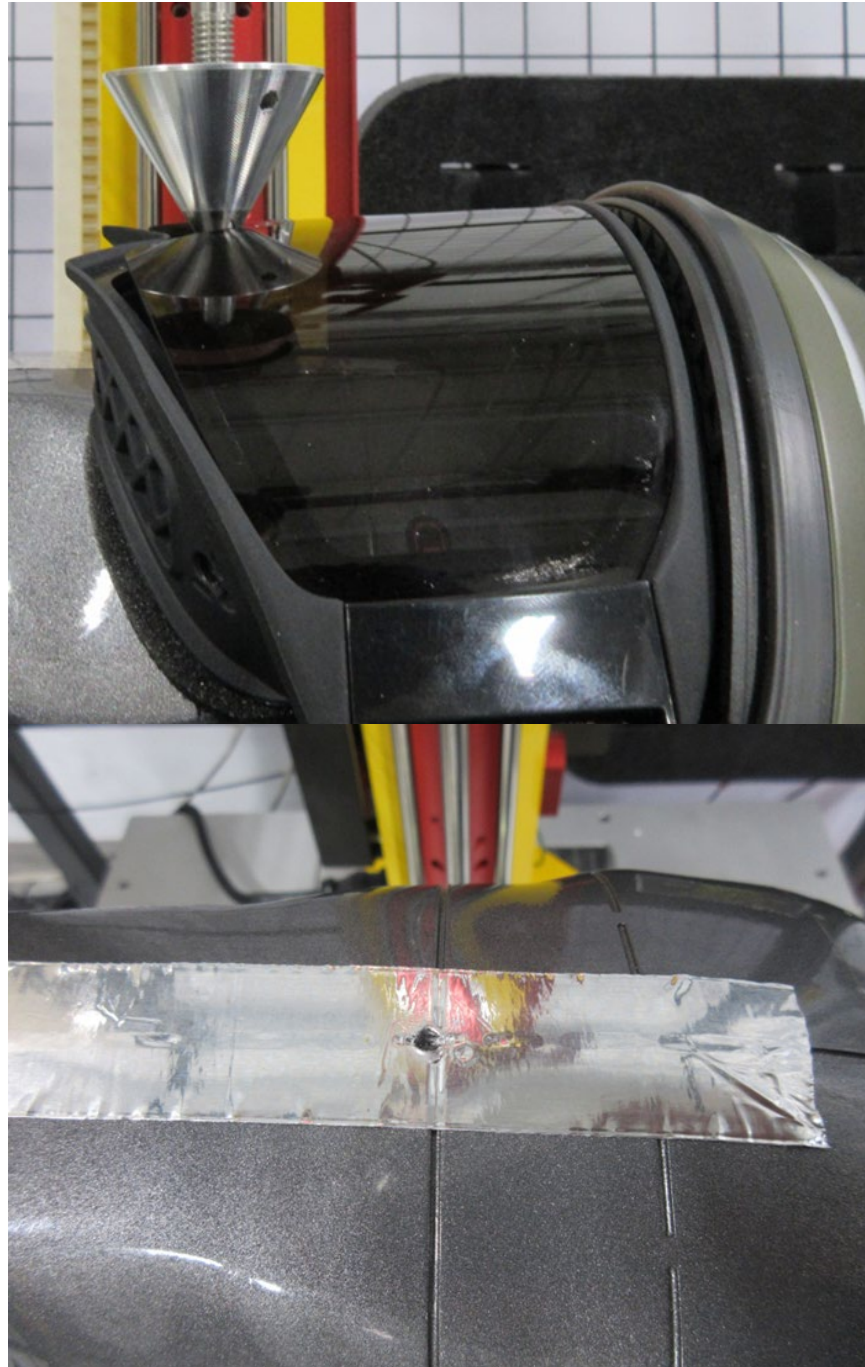
Figure 22. Shark Street Drak Face Shield Penetration Damage
