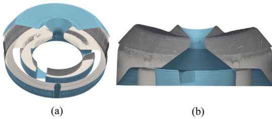
Fig. 1. 3-D reconstruction of the fuel nozzle: (a) isometric view and (b) side view [59].
