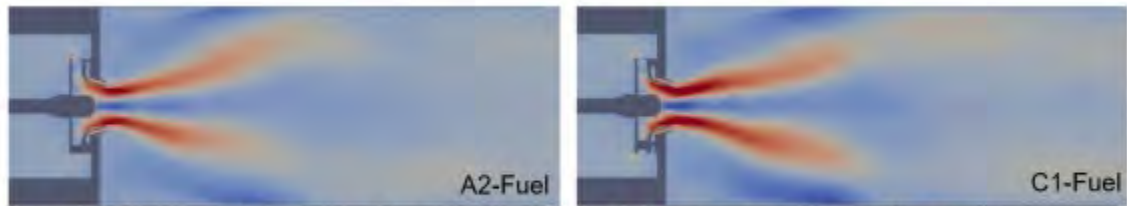
Figure 12: Contours of temperature from reacting LES of high shear rig combustor (top row) Instantaneous temperature contours (bottom row) mean or time-averaged temperature contours in central plane
