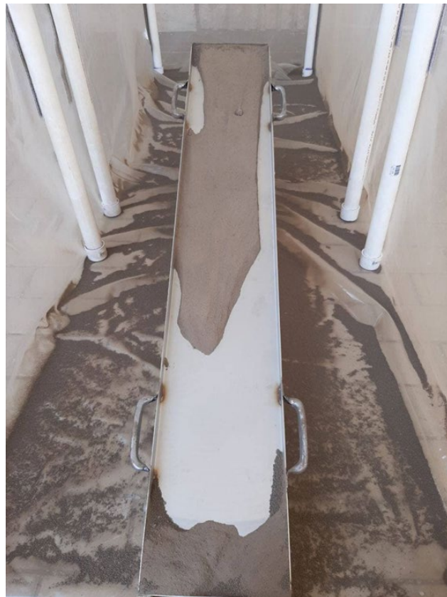
Figure 4.8: Photo of a Wind Erosion Test for a Sloped Configuration
