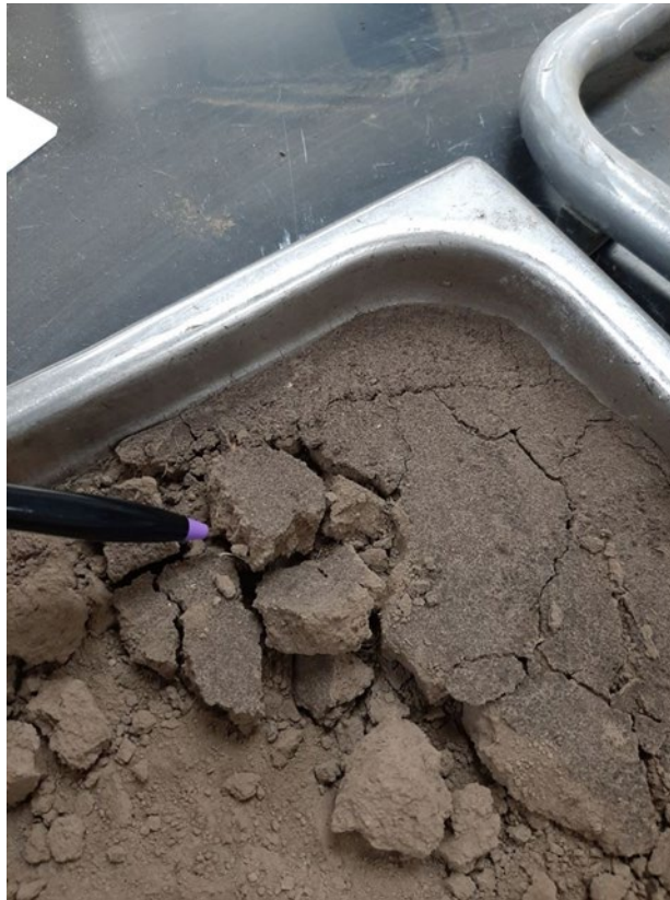
Figure 5.2: Crust Formation During Hand Penetrometer Tests for Spraying Rate of 0.0863 gal/ft 2
