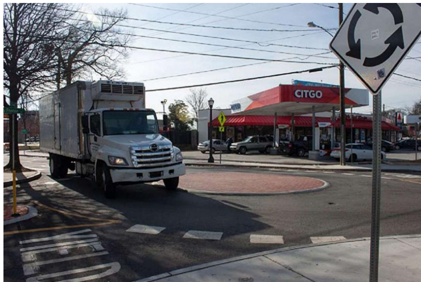
Figure 3.6 Mini-Roundabout (FHWA, 2018b)
