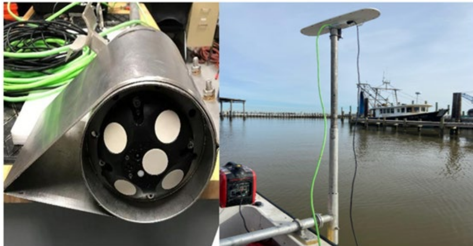
Figure 4. Photos of Signature 1000 ADCP inside teardrop enclosure (left) and GNSS antenna on top of side-mounted instrument pole (right).
