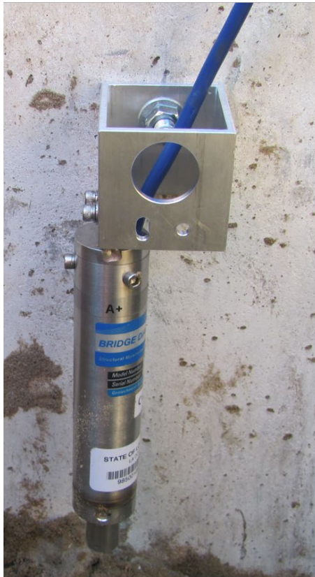
(c) Photo of the tiltmeter.
