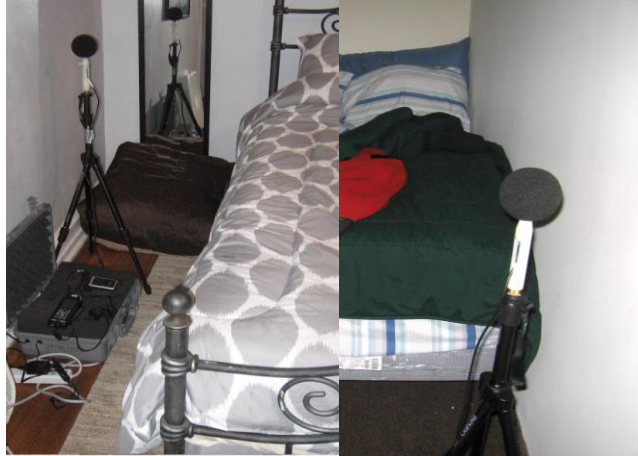
Figure 4.3: Examples of the placement of the indoor microphone near the sleeping position.
