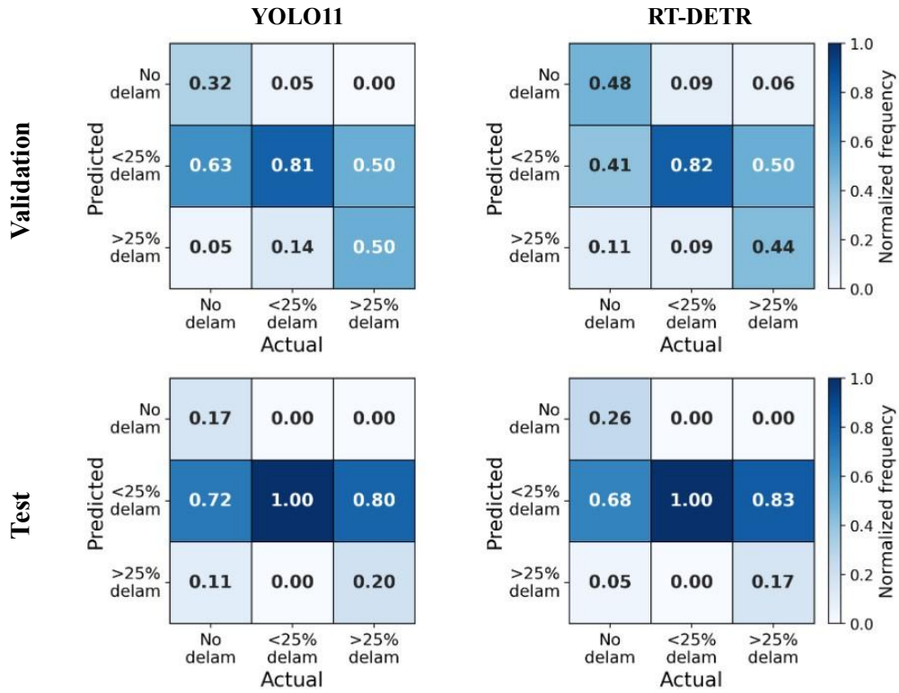
Figure 5.7: Normalized confusion matrix on validation and test set for delamination with YOLO and RT-DETR
