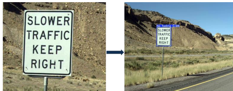
Figure 5.16: Fading effect due to peeling of letters
