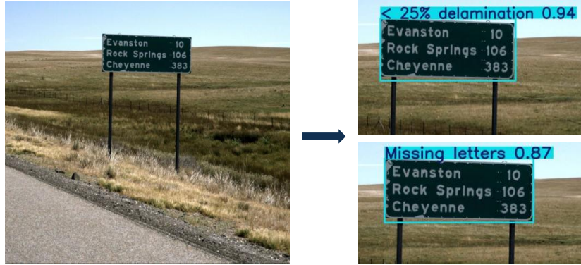
Figure 5.18: Delamination is present, but no missing letters
