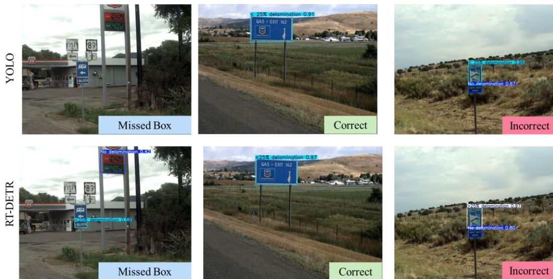
Figure 5.10: Representative inferences from YOLO11 and RT-DETR for delamination
