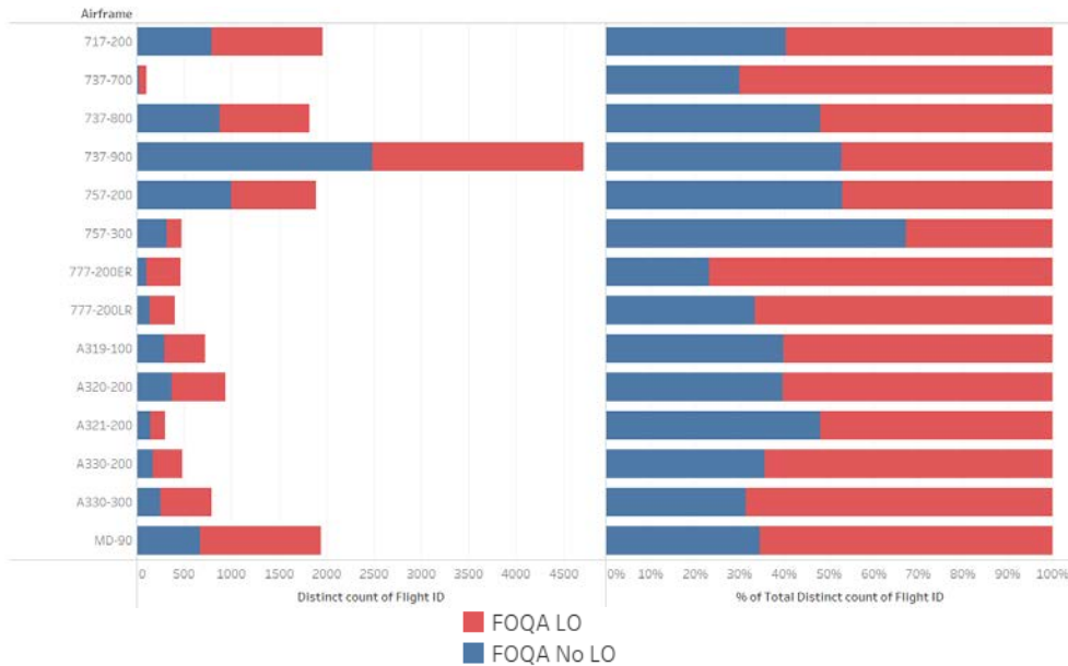
Figure 5. Level off percentage breakdown by aircraft including all 71 airports in the database.
