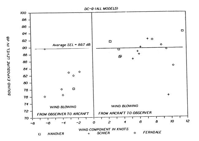
FIGURE 13. MEASURED SELS AS A FUNCTION OF WIND VELOCITY FOR DC9
