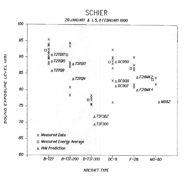
FIGURE 7. MEASURED SOUND EXPOSURE LEVELS AT 851 MAIN AVENUE
