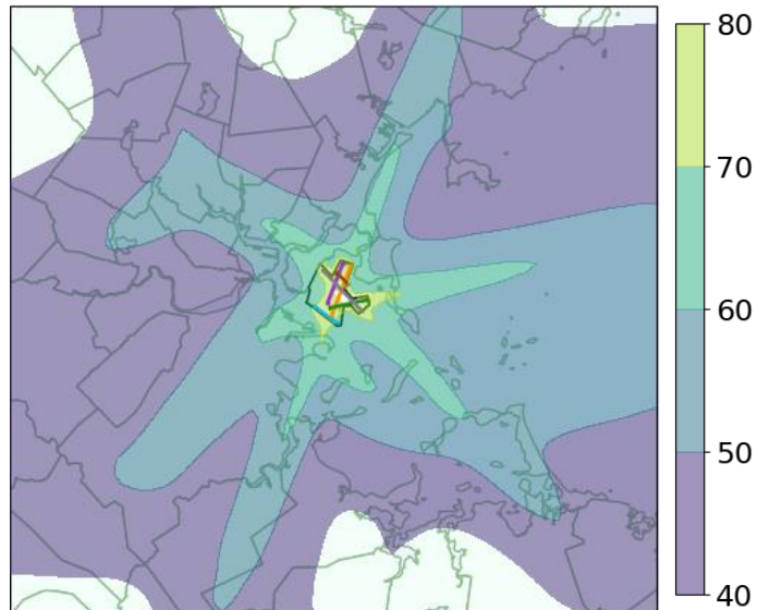
Figure 27. DNL for KBOS using data from 2016 computed on a 20 nmi x 20 nmi grid with 0.25 nmi grid spacing.
