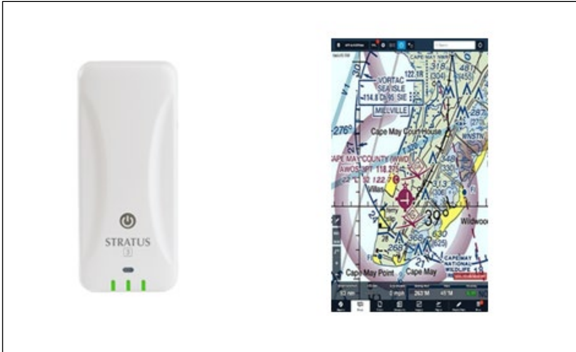
Figure 6. Appareo Stratus Portable ADS-B In Receiver (left) and ForeFlight EFB App, on iPad (right)
