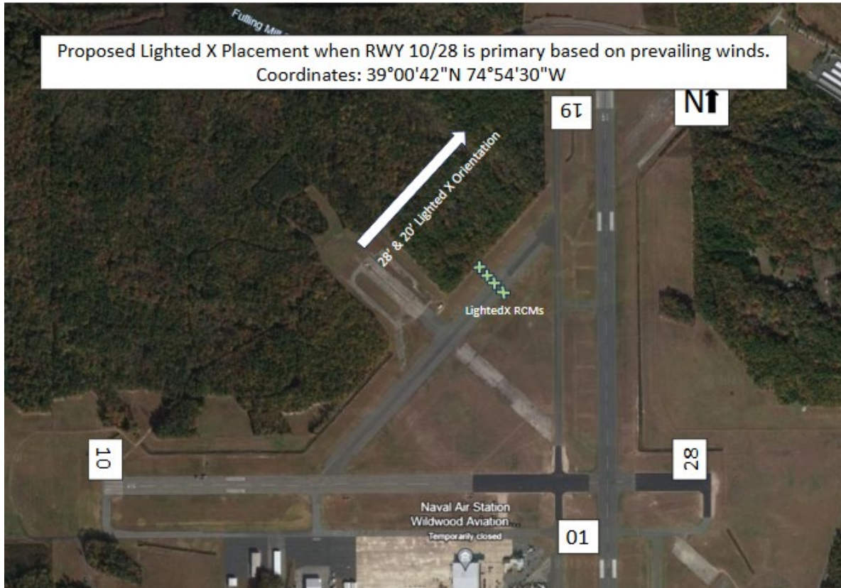
Figure 10. Lighted X Placement
