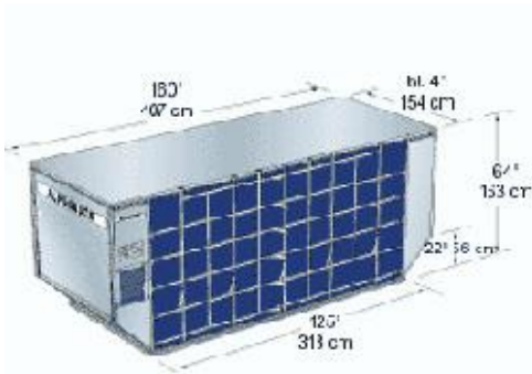
Exhibit 6-7: LD39/ALF Air Freight Container would fit the Quintero One
